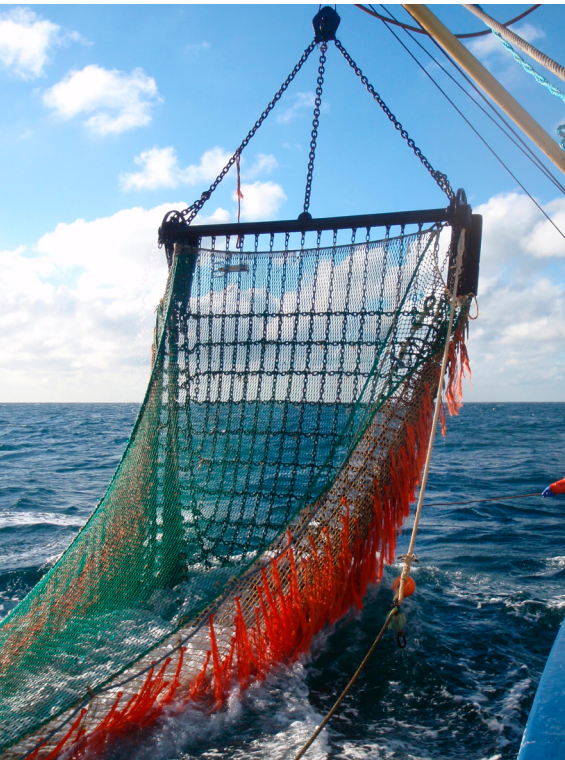
Figure 8: The retrieval of the port-side beam trawl. Note the attachment of the CTD unit to the underside of the header rope.
