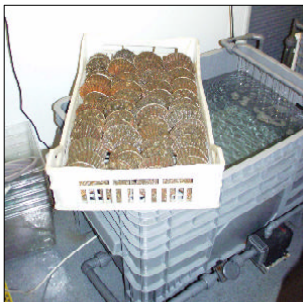
One of the CEFAS systems used for scallop depuration experiments
