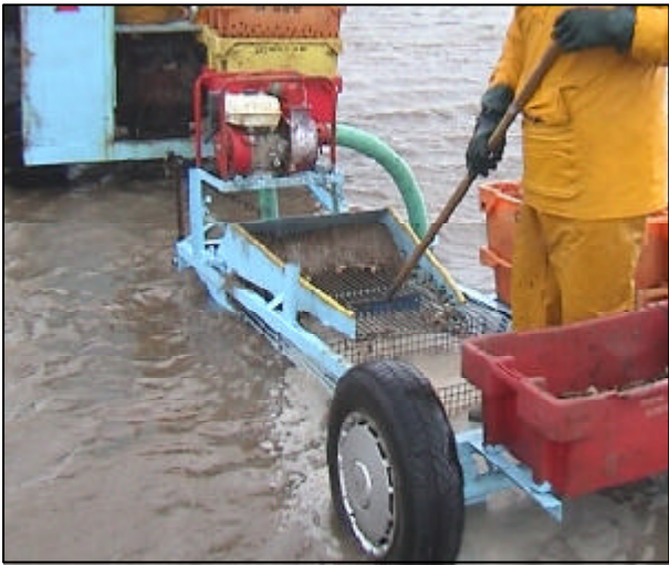
The cockle dredge, with an operator raking the catch from the sorting grid
