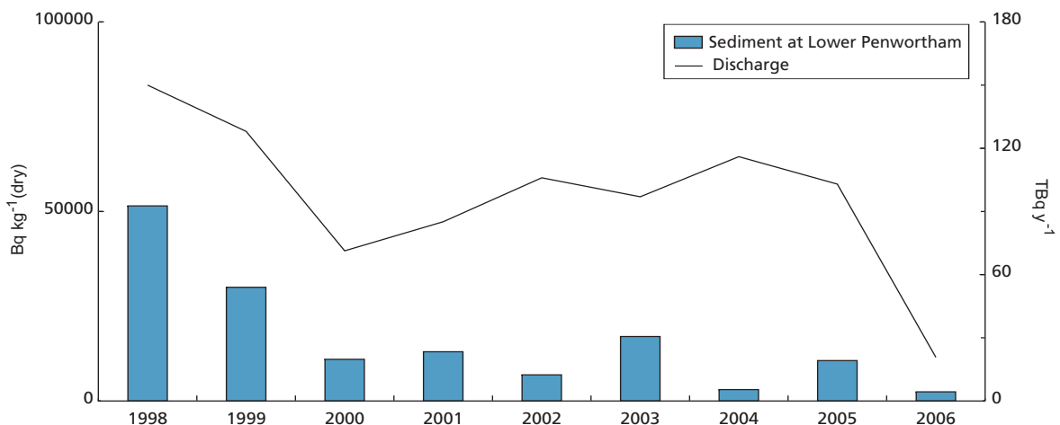
Figure 2.3. Total beta in liquid discharges from Springfields and concentrations in sediment at Lower Penwortham
