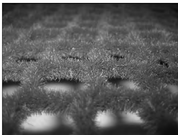
Aquaculture nets made with Dyneema® and the non-toxic Thorn-D® antifouling treatment (Photo DSM Dyneema, DYNPR068)
