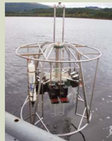
Figure 8 Bowers and Connolly megacore including barrels of an internal diameter of 100 mm
