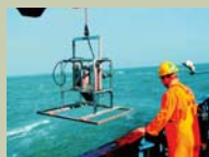
Figure 4. Cefas Sediment Profile Imagery (SPI) camera
