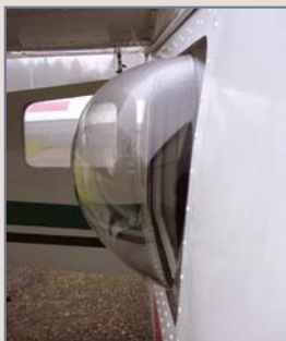
Figure 2: Bubble window, placed at both rear seats for unobstructed observation on the transect line.
