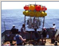
Figure 2a: Biogeochemical lander (IMPHIM)
