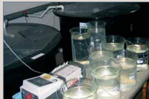
Dosing of tanks with a multichannel peristaltic pump
