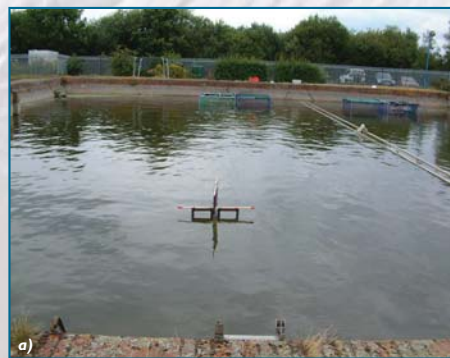
Figure 1: A free-standing detector array comprising eight individual PIT detector antennae; stands were constructed to allow full coverage of the water column within the trial lagoon.
