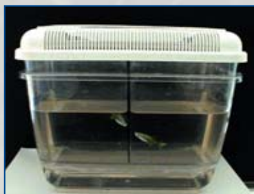
Experimental fish tank containing a pair of zebrafish separated by a perspex divider which is removed once a week to allow mating.
