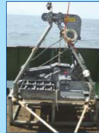
Figure 5: Hamon grab mounted with video and lights with an example of macrofauna and a typical grab sample
