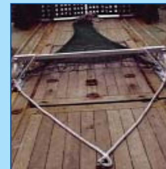
Figure 6: Heavy duty 2m beam trawl with examples of beam trawl samples collected from an area of high dredging intensity and a reference location
