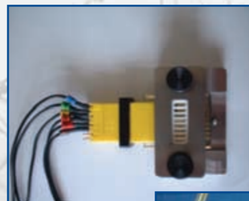
Figure 4a: Array of gold electrodes evaporated onto glass substrate clamped into small volume incubation chamber.
