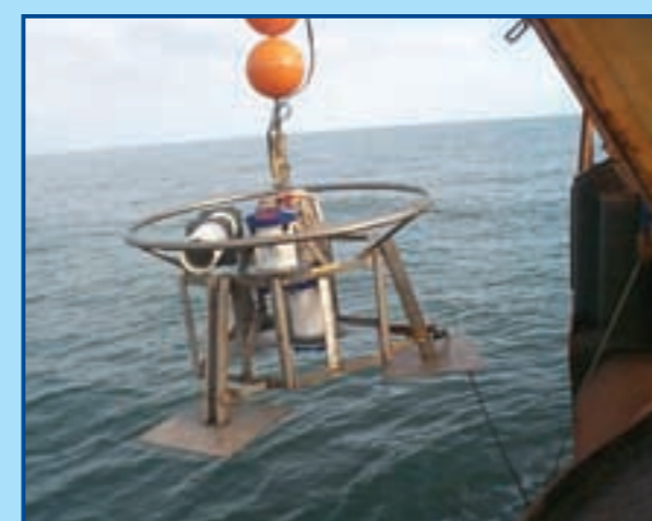
Figure 4: Simplified Lander Assembly (CEFAS ADCP frame)
