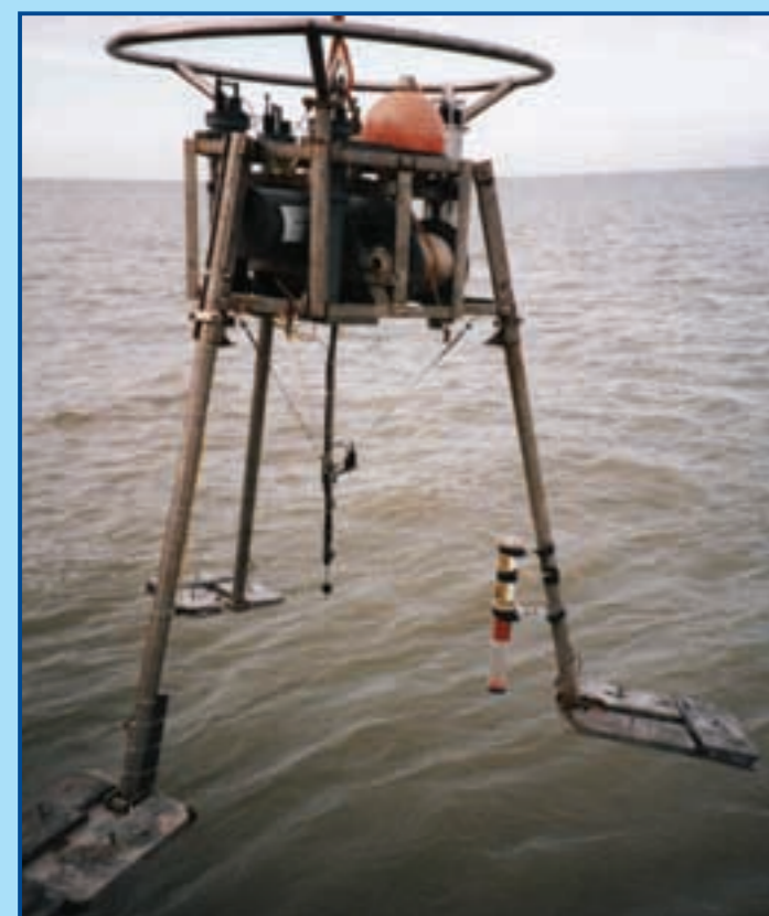
Figure 1: Lander interface interactions (when on bed) CEFAS Minipod Lander - for measuring near-bed flows and suspended sediment behaviour
