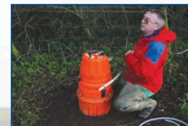
Figure 5: Automated sampling apparatus for storm surveys.
