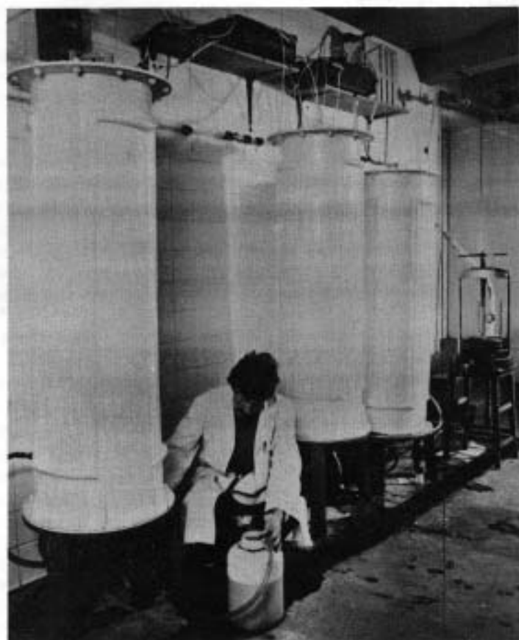
Figure1 The 200 l internally illuminated algal vessels. Note the configuration of the cooling element.
