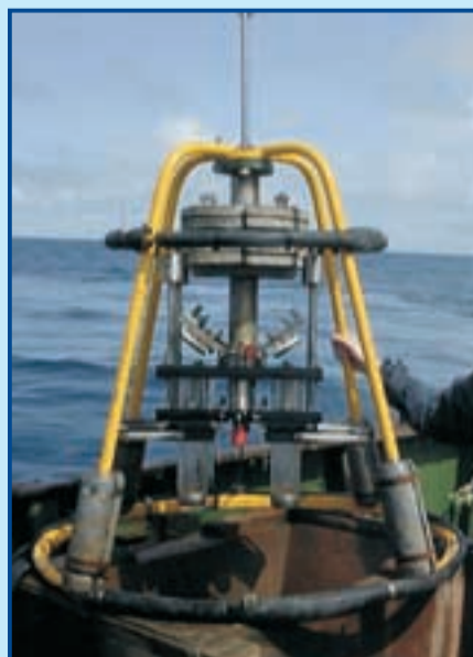
Figure 3: Bowers and Connelly Multiple Mini-Corer
