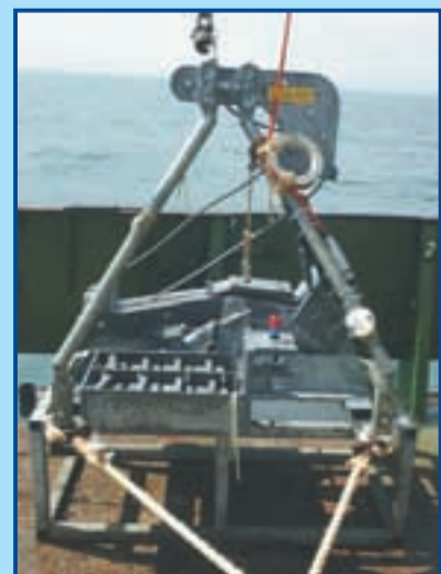
Figure 4: Hamon grab with video and light attached
