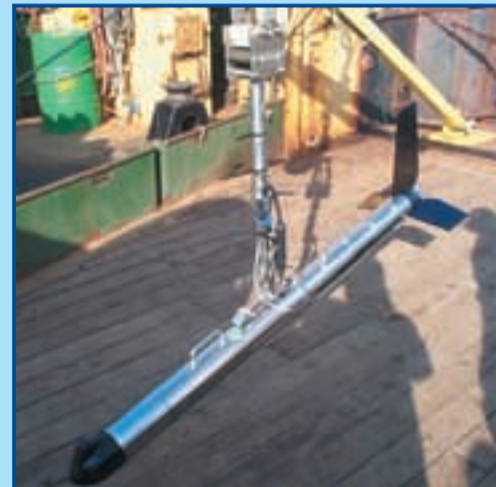
Figure 2: Datasonics digital chirps sidescan sonar fish
