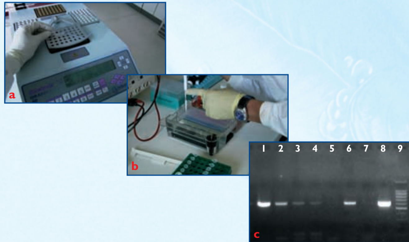
Detection of virus nucleic acid by PCR. Amplification of virus sequences using a robot thermocycler (a). Agarose gel electrophoresis of PCR products (b). Visualisation of amplified virus sequences as white bands on the gel (c).
