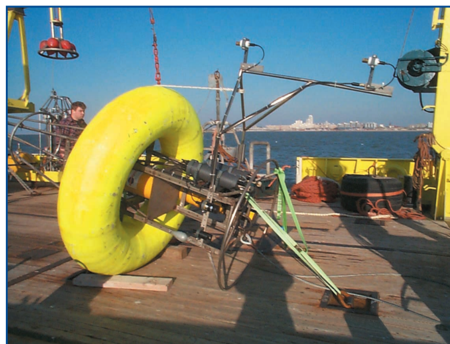
Figure 2a SmartBuoy with a range of sensors before deployment. (photo D. Sivyer)
