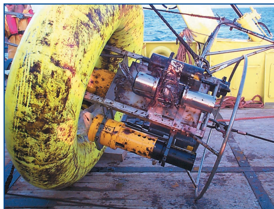
Figure 2b SmartBuoy with a range of sensors after recovery. (photo D. Sivyer)
