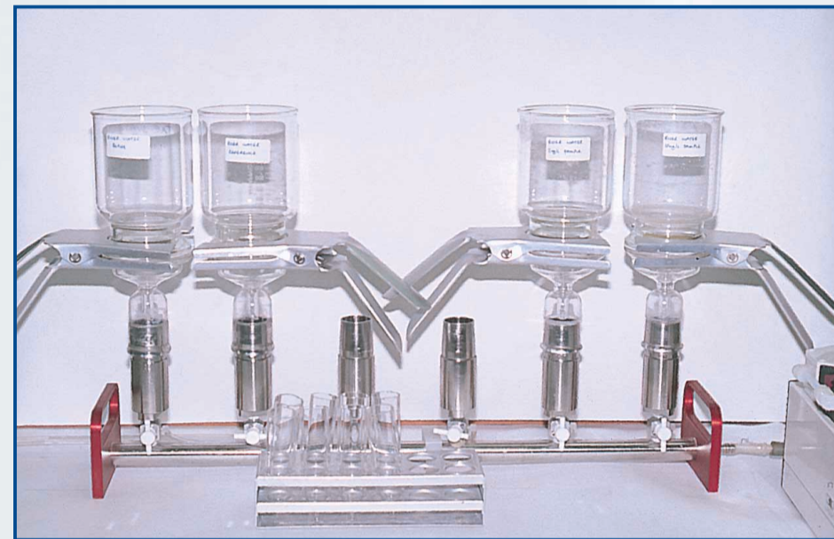
The experimental set-up for disk extraction manifold
