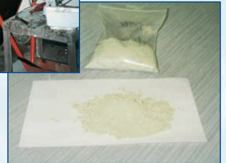
The Laboratory Spray-Drier and an example of the algae powder produced (Tetraselmis).
