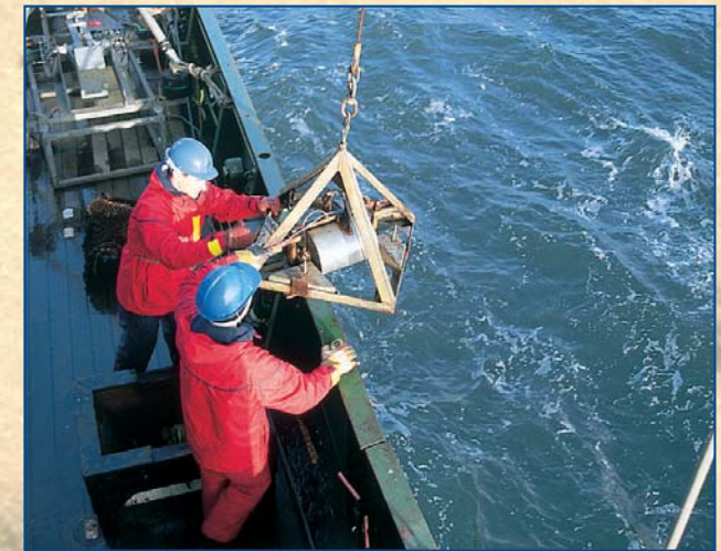
Collecting a sediment sample with the Day grab.
