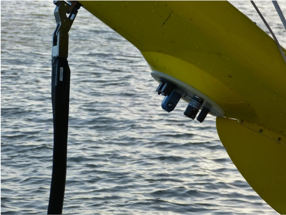
Figure 2: Cefas SmartBuoy sensors fitted to the ADCP cavity
