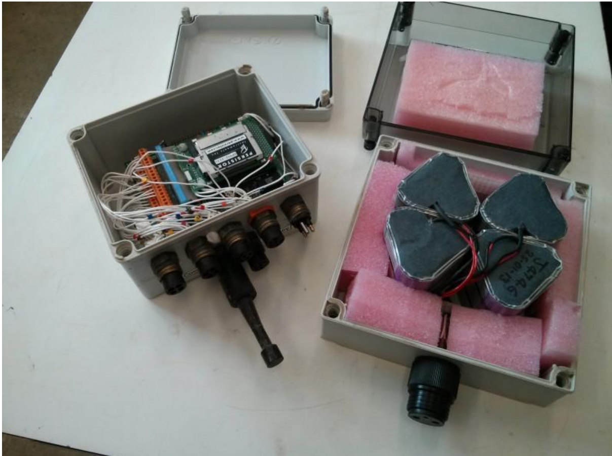
Figure 1: ESM-2 and lithium battery pack in custom housings
