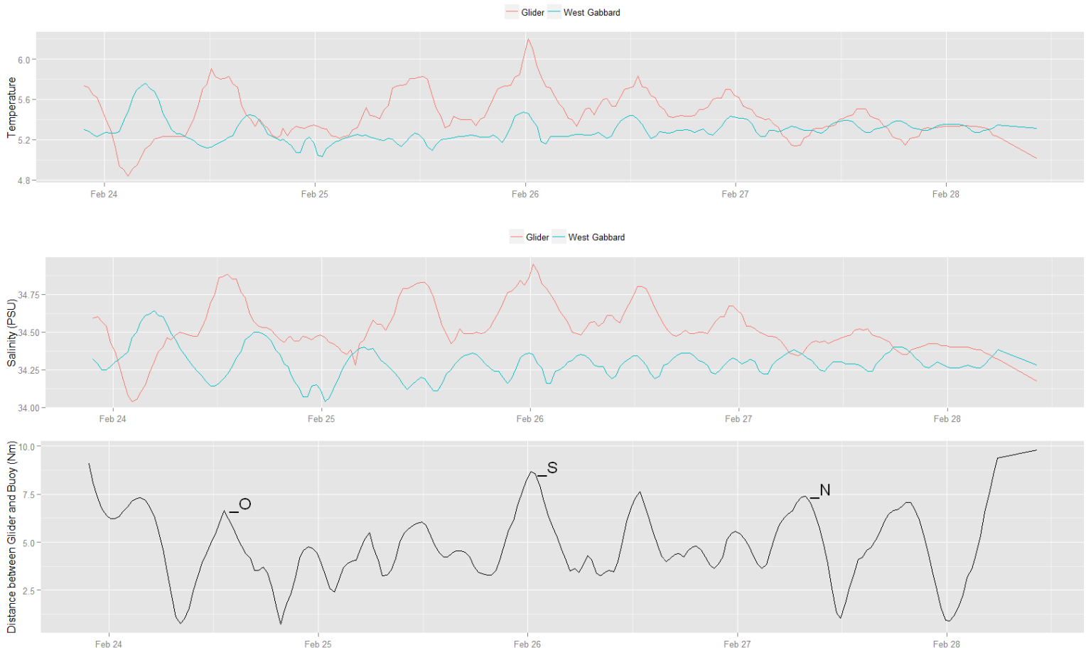
Fig. 9: Wave Glider and West Gabbard data; (a) salinity, (b) temperature with (c) distance of Wave Glider from West Gabbard buoy
