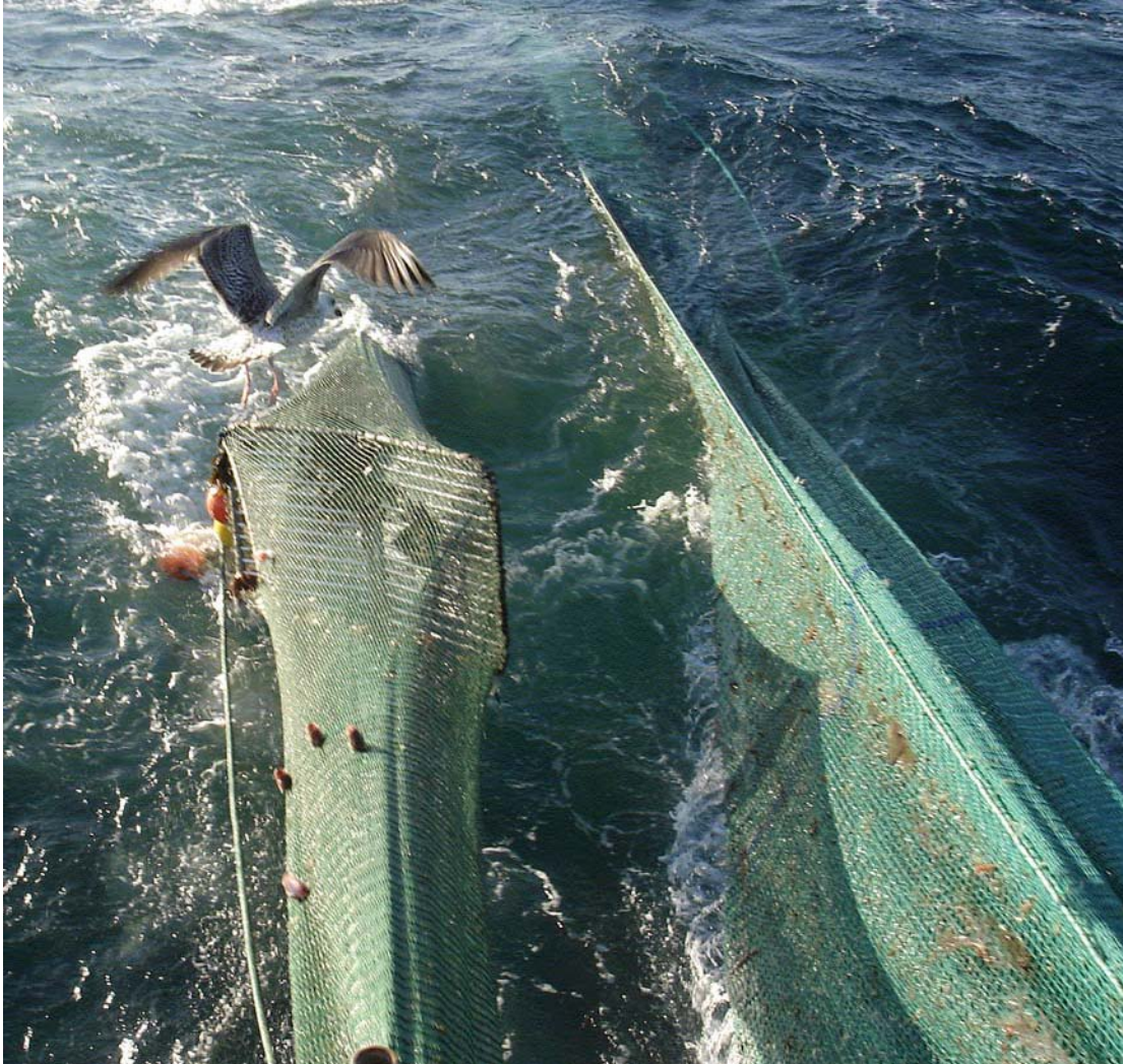
Figure 2. The twin-rig trial method: twin-rigged trawling with a standard trawl on the portside and a Swedish grid on the starboard side
