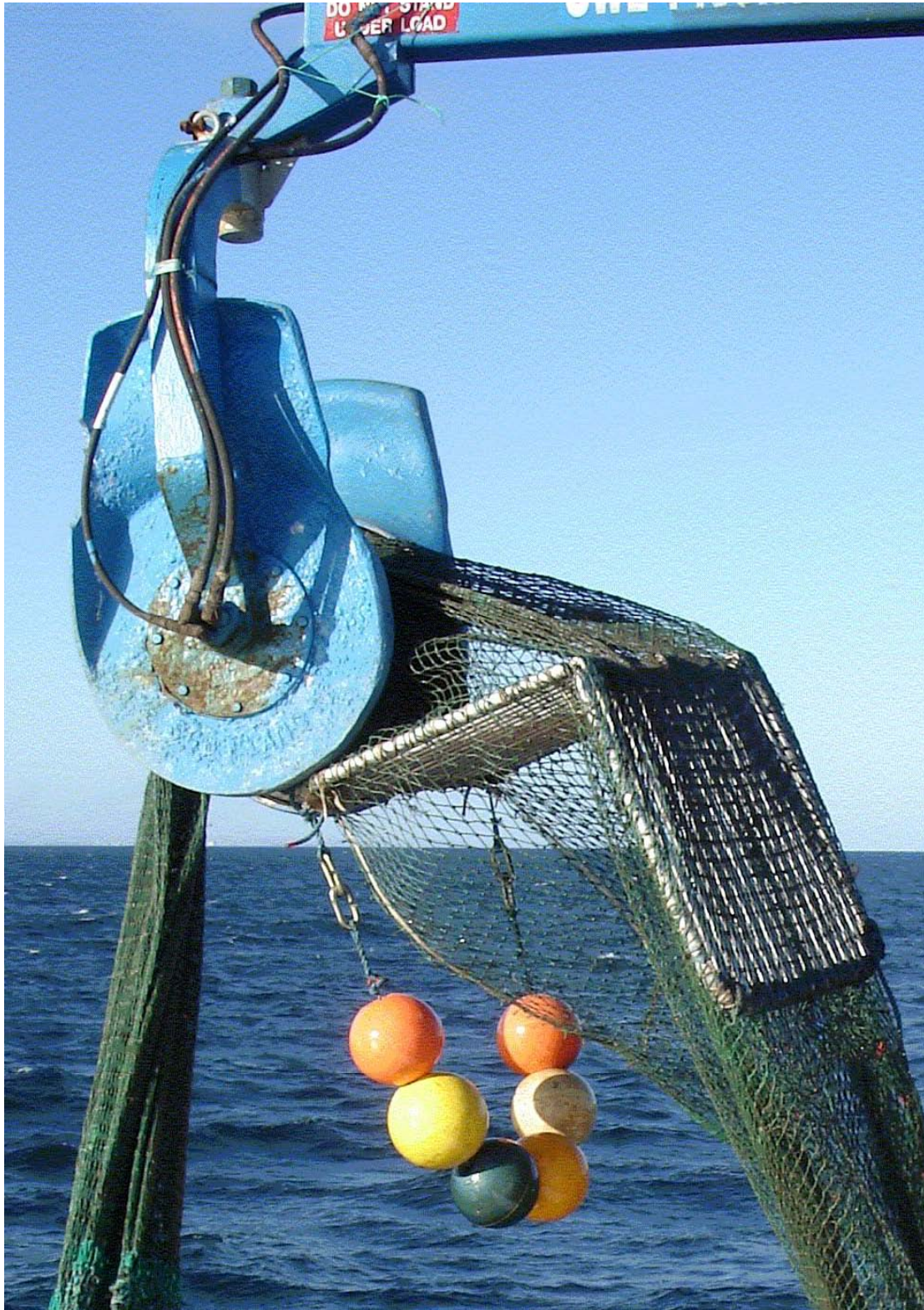
Figure 3. Using the power block to manoeuvre the Swedish grid during hauling, note the grid does not pass through the power block
