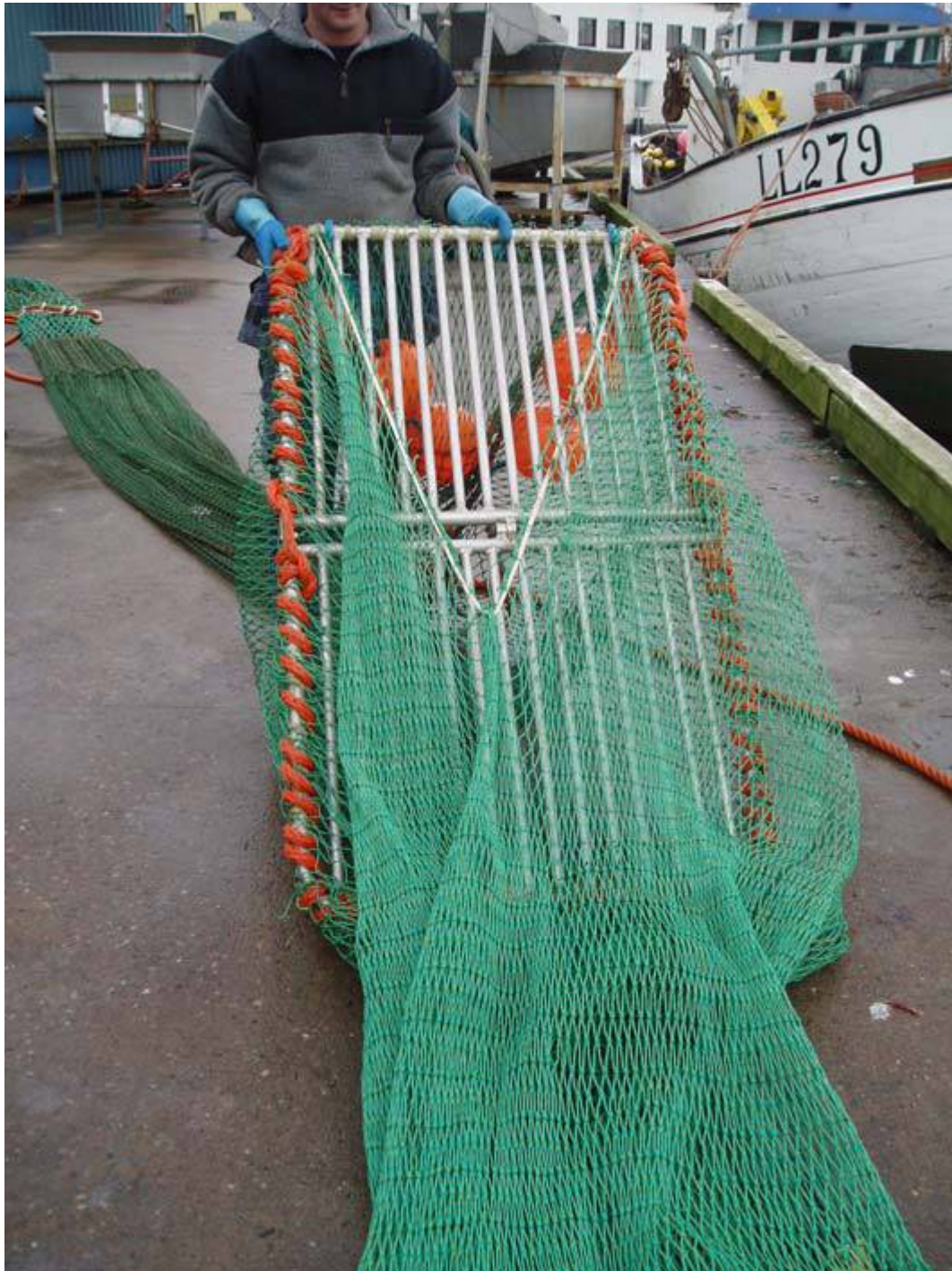
Figure 1 A typical grid used in the Swedish fishery. Large fish are guided out of the trawl by the grid while smaller fish and Nephrops pass through the grid and enter the codend. The grid is made of aluminum and is jointed to facilitate winding the trawl on to the net drum
