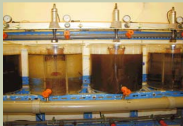
Figure 2. A standard Sea Test in process. The difference can clearly be noted between mechanically dispersed oil (left) and chemically dispersed oil (right).
