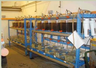
Figure 1. The statutory Sea Test rig set-up as used for the toxicity assessment of oil spill treatment products in the United Kingdom.
