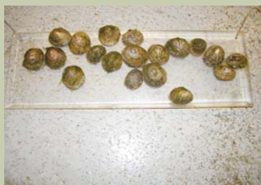
Figure 3. The common limpet ( Patella vulgata ) is used in the standard Rocky Shore Test. Here the test organisms are seen on the Perspex plate prior to oil or product treatment.
