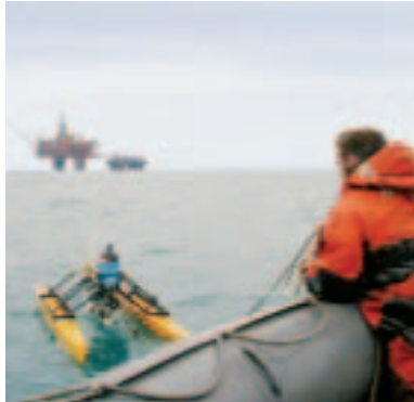
Above and left page: Collecting Sea Surface Microlayer Samples around the Statfjord oil field
