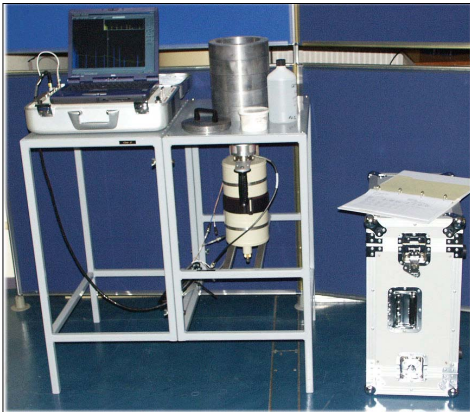
Perkin-Elmer HpGe detector assembled for use.
