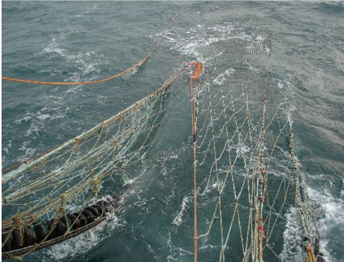
The Eliminator trawl being hauled aboard the MFV Our Lass II in the North Sea trials Dec 2007 (NB: large rope meshes of 2.4 metres at front and in belly of trawl)
