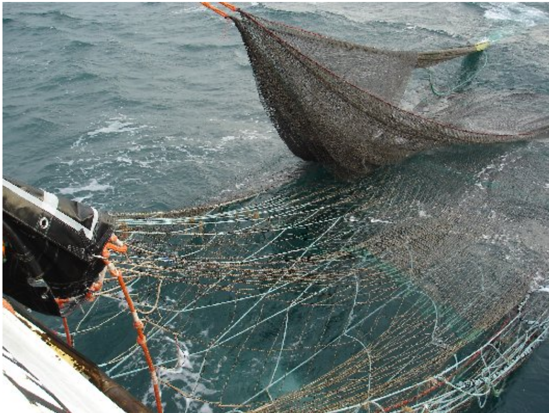
The Eliminator trawl being hauled aboard the MFV Our Lass II in the North Sea trials Dec 2007 (NB: large rope meshes of 2.4 metres at front of trawl)
