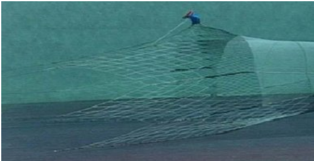
The Eliminator trawl in earlier Canadian flume tank trials (Courtesy of Superior Trawls, USA)
