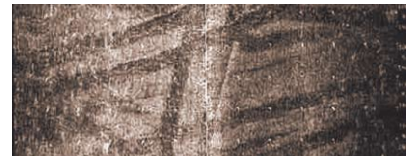
Sidescan image of beam trawl scars on the seabed
