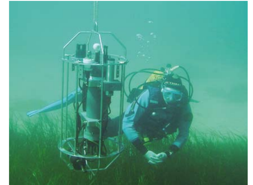
Above: The Cefas profiler, being deployed over a seagrass bed
