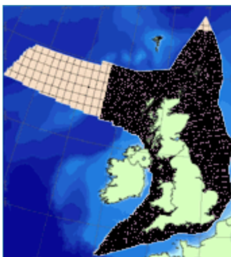
Figure 2a. The location of the wave and wind model grids, as used in the Met Office Global and UK Models. These have a spatial resolution of 60 km and 12 km respectively
