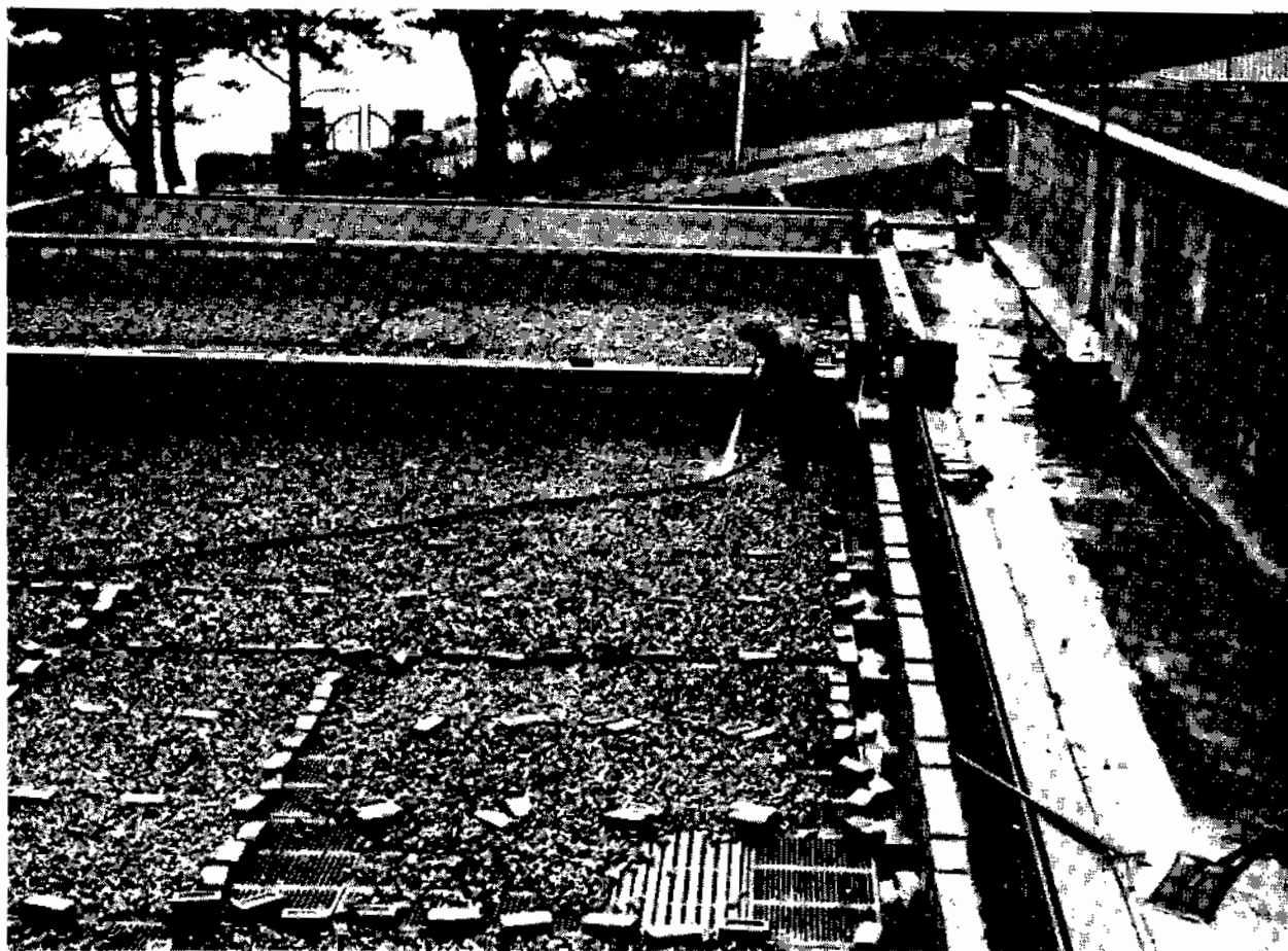
Plate 4 Mussel-cleansing tanks at Conway, showing mussels being hosed, and the supporting grids. On the right can be seen the gutter and penstocks used when flushing the bottom of the tank.
