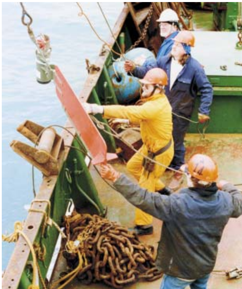
Laying current meters
