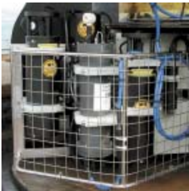
CEFAS instrumentation package below the surface, attached to the ODAS buoy
