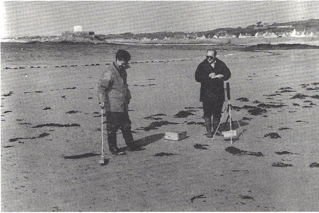
Figure 9. Taking close-contact beta plus gamma dose measurements (on left) and gamma dose measurements in air (on right) at Rocquaine Bay beach Guernsey
