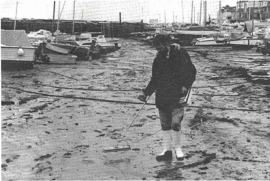
Figure 11. Checking for particulate activity in St Aubin's harbour, Jersey using a close-contact beta plus gamma detector
