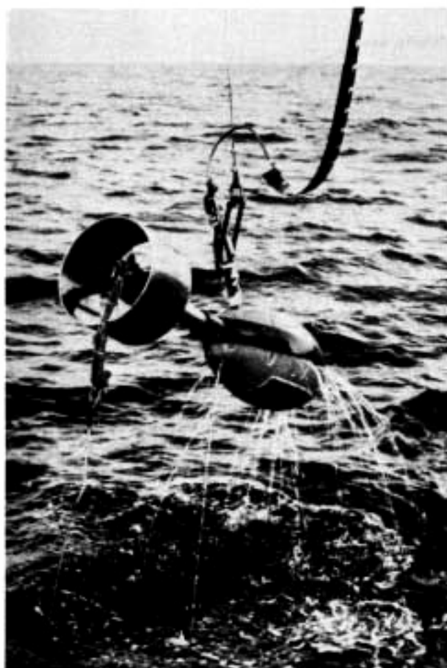
Figure 10 Towed body and towing cable. The towed body is being recovered on a separate wire rope.
