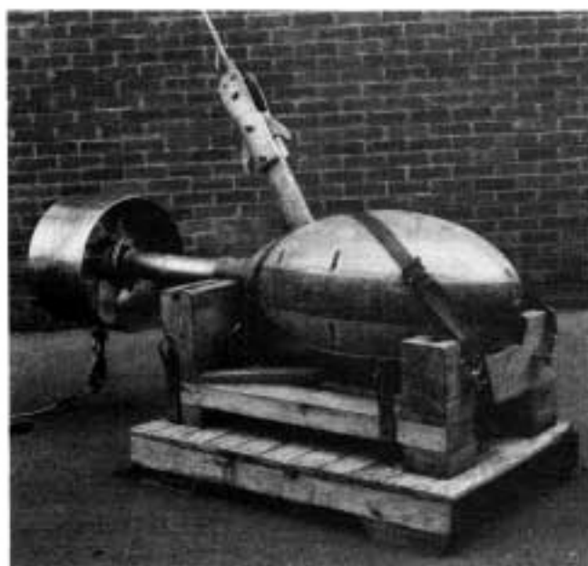
Figure 4 Towed body and cradle. The transducer fitted inside the towed body transmits and receives through an acoustically-transparent window (just visible in the under-surface). A line is attached to the tail as a safety precaution in case the towing cable fails during survey. The cradle is necessary both as protective stowage at sea and as a lifting frame when the body is craned between ship and shore.
