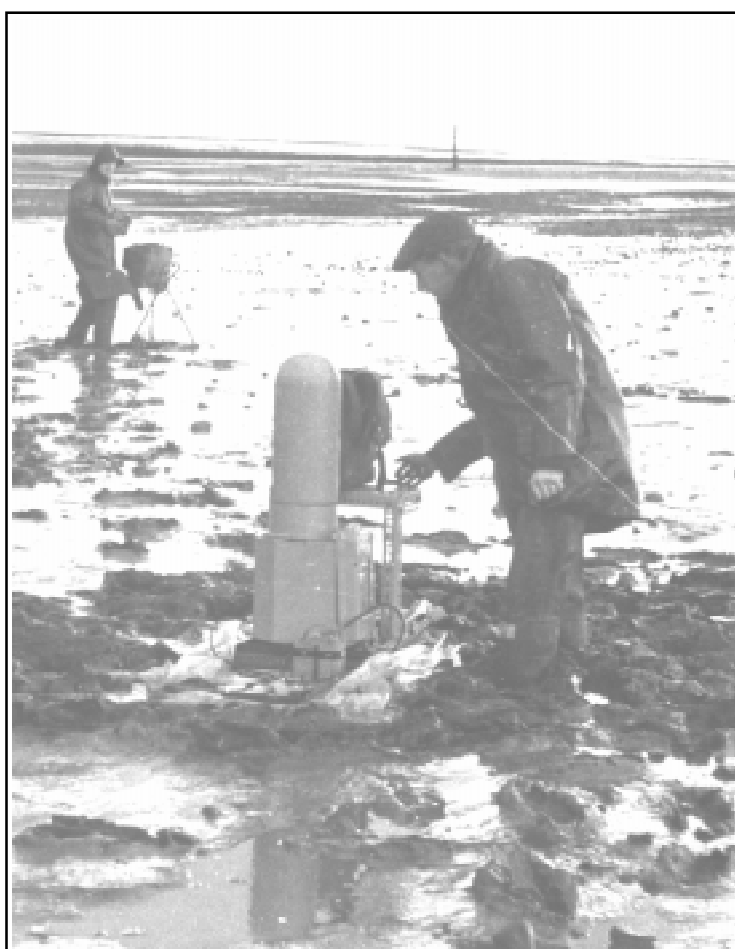
Figure 6. Ken Firman (left) with 'Airmec' GM counter and Alan Moore with 'Gammagraph' high-pressure ionisation chamber, near Lytham, circa 1963
